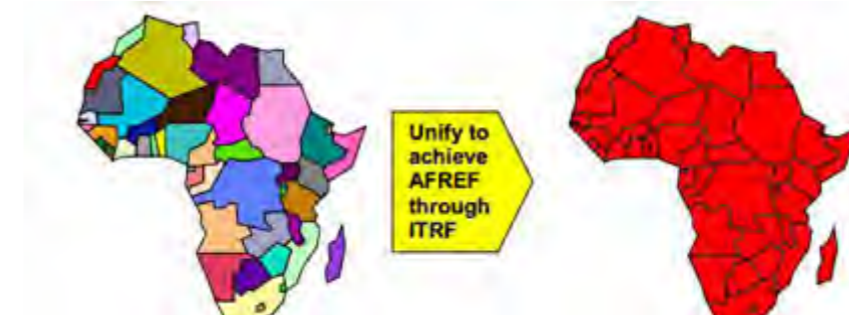
Figure 5: AFREF is conceived as unifying the national reference frames of Africa into a common reference frame for the continent.
