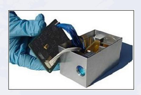
Argus is a miniature technology demonstration instrument, the objective is to detect greenhouse gas constituents in the near infrared region using Earthshine spectra. Argus features only an along-track footprint of 1km x 1km (there is no scan capability in cross-track). Initial tests will be carried out to detect pollution plumes of industrial origin. Argus has demonstrated and validated the detection
