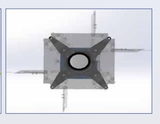
The antenna module on the nadir plane of the satellite must have a hole for the lens of the camera payload to pass through. As no hardware is yet determined for the payload, assumptions has to be made regarding this hole. One possibility is to have the hole centered such that the lens passes through the
