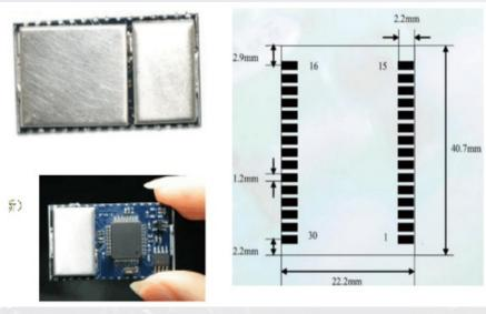
BMOS2-100(thumb machine) Satellite Navigation receiver is a BD/GPS receiver by which we can realize the switch between GPS and BD navigation without hardware update. BMOS2-100 highly integrate RF, baseband processing and positioning software, thus can provide high accuracy data of three-dimensional position, velocity and time, as well as original observation data, etc. The thumb machine has the charac-
